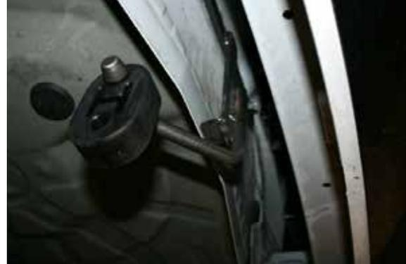
**Step 6:** Using the original gasket (Replace if necessary), install the Takeda Mid Pipe by sliding the rubber hanger mount onto the chassis and using the original (x2) bolts removed from step 2 and the supplied (x2) nuts and tighten.
